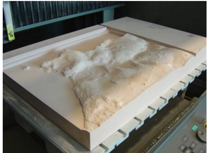
Lower Red River model after first Cut
