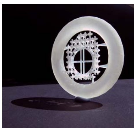
20, 21& 22 CAD Visualisation of a ring ,Wax RP model for casting, final silver ring
